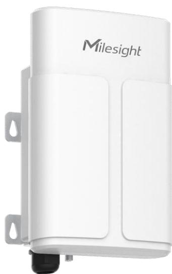
UG67 is a robust 8-channel outdoor LoRaWAN<sup>®</sup> gateway. Adopting SX1302 LoRa chip and high-performance quad-core CPU, UG67 supports connection with more than 2000 nodes. UG67 has line of sight up to 15 km and IP67 waterproof case, which is ideally suited to smart agriculture, smart metering and many other outdoor applications.
